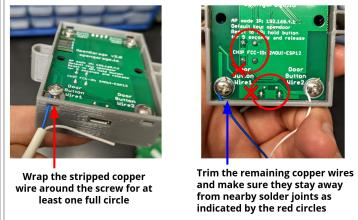
o Insert the other end of the stripped wires to the door button terminal you located above. Because OpenGarage uses a relay to simulate button click, **the two wires have no polarity**.
